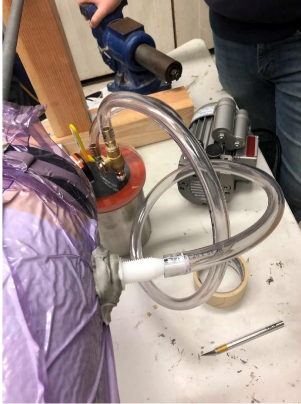
Figure 7. Vacuum pump configuration while putting the vacuum on the tube
