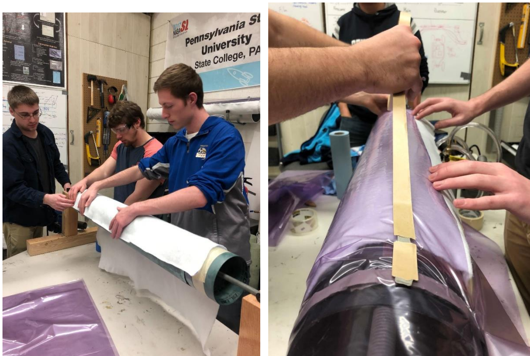
Figure 6. Wrapping the carbon fiber with nylon release and breather cloth layers and sealing the nylon bagging with sealant tape
