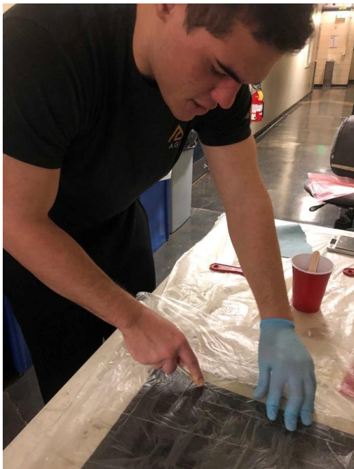
Figure 3. Cutting Carbon Fiber Plies
