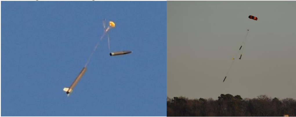
Figure 51. Parachute descent under drogue (left) and main (main) during vehicle demonstration flight
