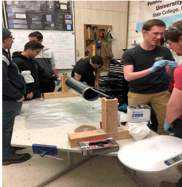
Figure 5. Carbon fiber plies wrapped around mandrel
