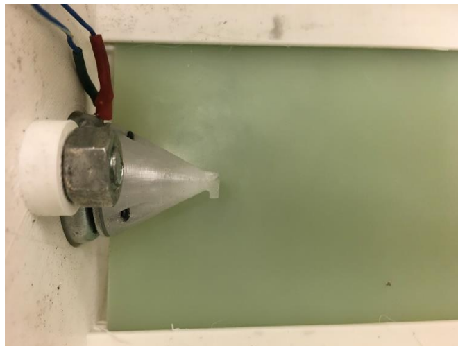
Figure 59. Solenoid Locking Mechanism for Rover Retainment
