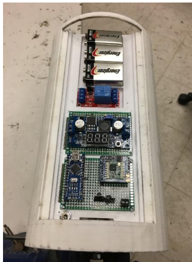
Figure 56. Electronics for Payload Deployment
