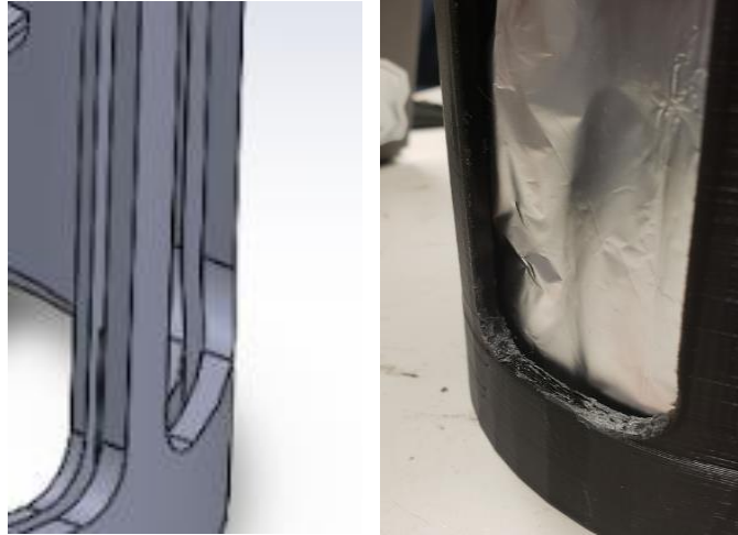
Figure 24. Faraday cage slots in SolidWorks model (left) and constructed avionics bay (right)
