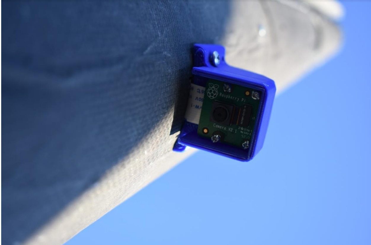
Figure 16. Assembled camera system on launch vehicle before fullscale test flight
