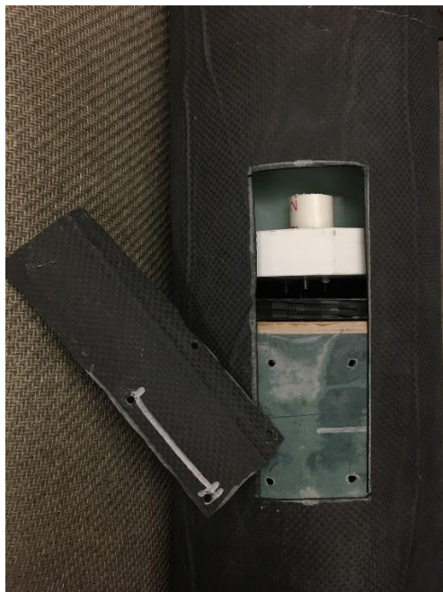
Figure 52. Payload Black Powder Charge Assembly with Door
