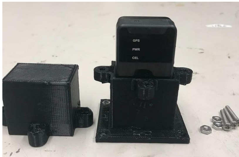
Figure 33. GPS in 3D Printed Bracket
