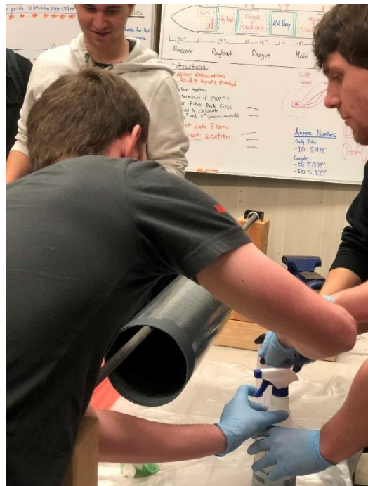
Figure 4. Blue tube mandrel wrapped in packing tape prior to carbon fiber wrapping
